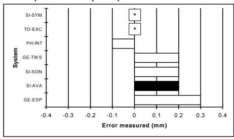
The optimum value is  $0 \pm 0.3$  mm. Systems are ranked in order of the absolute deviation from optimum. \*The system has the optimum measured error value of 0.0 mm.
