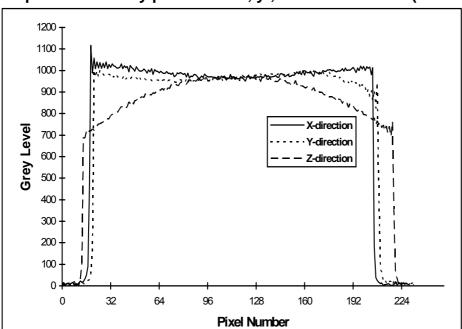
Graph 3: Uniformity profiles in x-, y-, and z- directions (unfiltered)
